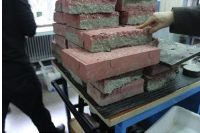
Figure II-71 Concrete blocks made partially by recycled aggregates
