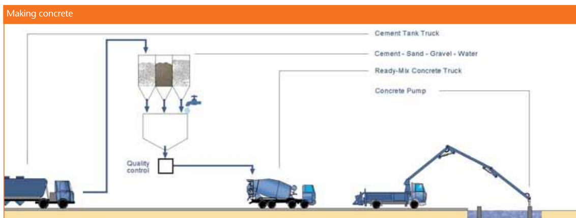
Figure I-1 Concrete Making Process (The Cement Sustainability Initiative)
