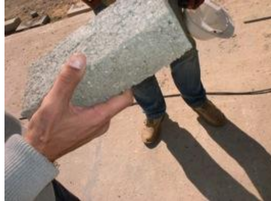
Figure VI-1 Concrete bricks produced from recycled concrete (Case study)
