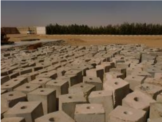
Figure VI-3 Concrete curb stones produced from recycled concrete (Case study)
